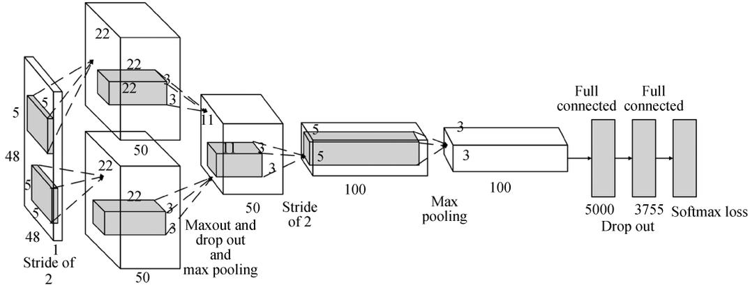
Fig. 1. Basic structure of our CNN model. (Notice that pooling layer is integrated into convolution layer)
